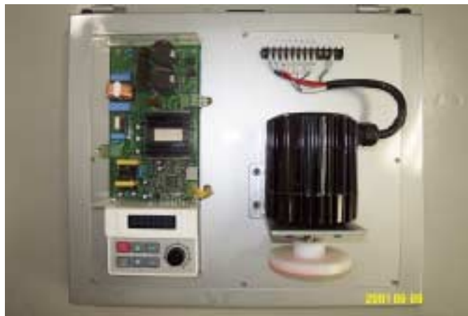
(b) Control board with BLDC motor
