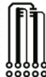
b. 175\text{ }^\circ\text{C/W} when mounted on a minimum pad of 2 oz copper
