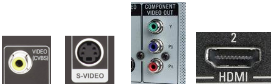
Figure 3: Typical video out connection schemes
