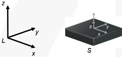
Figure 1. FIS1100 aligned with Local coordinate frame (L). The orientation of the FIS1100 is identified by pin1, indicated by the small grey dot on the FIS1100 sensor (S).
