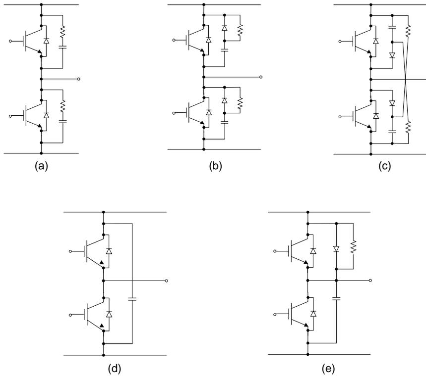
Fig. 11. Scheme of each type of snubber circuit
