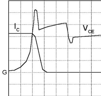
Fig. 10. Turn-off waveform of IGBT with snubber
