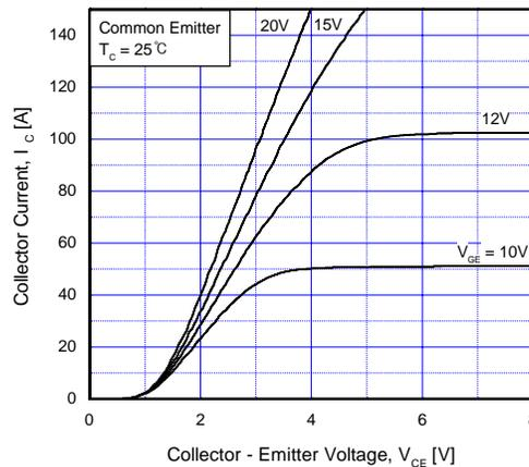
Fig. 4. Fairchild SGL50N60RUF D Typical Output Characteristics
