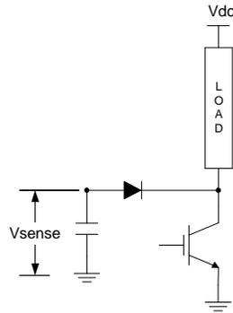
Fig. 8. Short-circuit sensing circuit using de-saturation method
