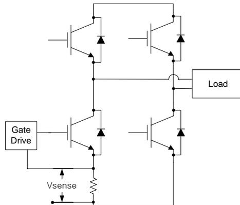
Fig. 6. Short-circuit sensing circuit with a sensing resistor
