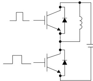
Fig. 2. Fault under load test circuit
